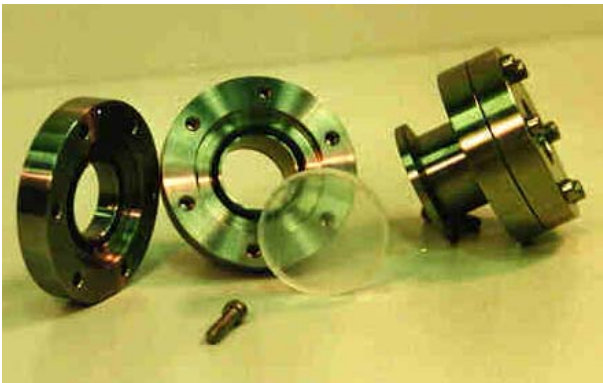
Fig 9. The cell windows have been mounted into the frames. When the window is changed, the whole frame is changed. Quick fixing of the frames is made with DN25KF flanges.
