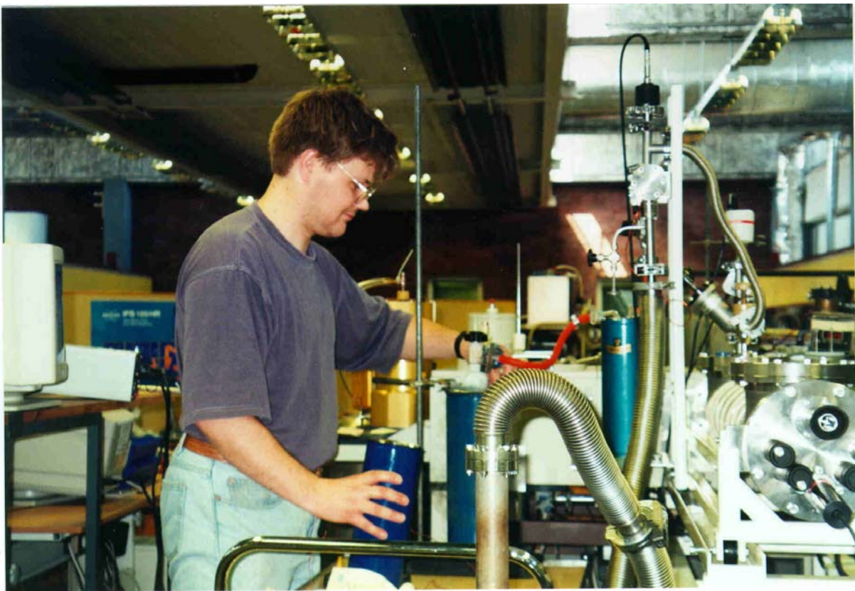
Fig 15. The cell is ready for measurements in Lund. Mr. Schroderus is preparing the first high resolution measurement with synchrotron radiation of torsional band of methyl-silane.
